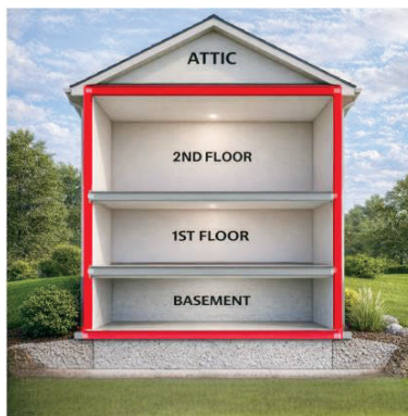
Figure 211-1: Diagram of Thermal Boundary
