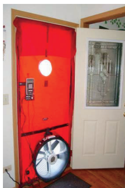
Figure 111-2-1: Blower door set-up
