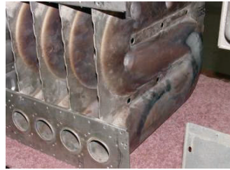
Figure 315-1-1: Furnace heat exchanger
