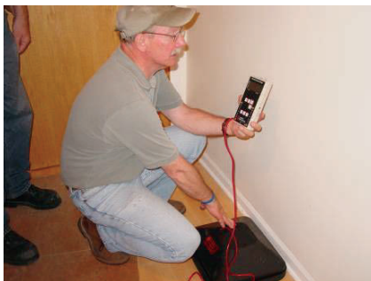
Figure 114-1: Pressure pan test
