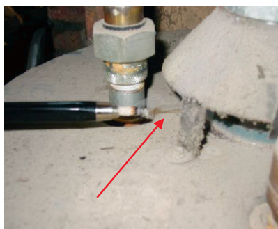
Figure 117-1: Conducting a spillage test with a smoke pencil
