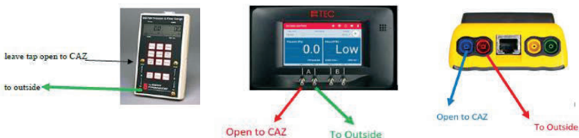
Figure 312-1-1-1 DG700, DG1000 & DM32 manometers set-up for WCD test. Note that hose to CAZ not necessary if readings are being taken in the CAZ
