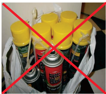
Figure 212-4-2-2: 1-part spray foam dispensed through a plastic straw is not permitted in the Weatherization Program
